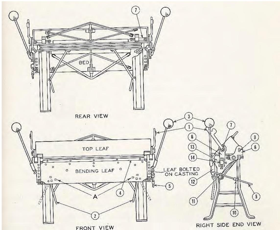
The 3 major parts of the brake are the bed, top leaf and bending leaf (shown in the front and rear views).
