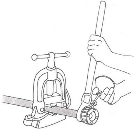
**Step 5.** While cutting threads, use generous amounts of oil. Chips may stop threader. Back off, brush chips away.
