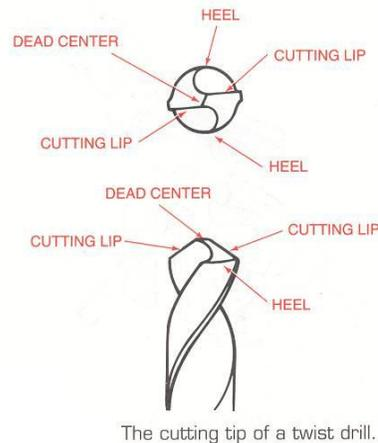
The cutting tip of a twist drill.
