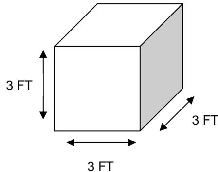
1. Determine the cubic yards of concrete needed by multiplying the thickness by the width and length:
