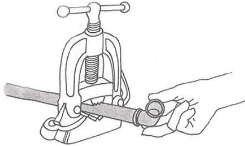
**Step 7.** Clean out the threaded inside of fitting; then screw it onto the pipe end by hand as far as it will go.
