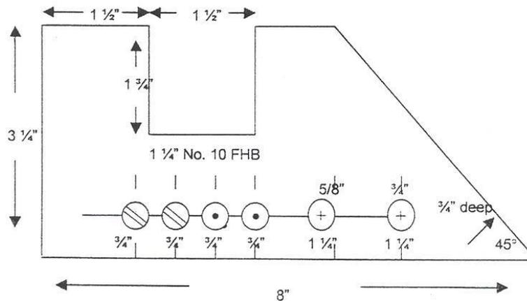
1. Mark slot with combination square according to dimensions.
