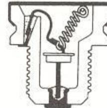
A typical Type-S non-tamperable fuse, and its adapter. Once an adapter has been screwed into a fuse-holder, it cannot be removed. This prevents the use of fuses larger than originally intended.
