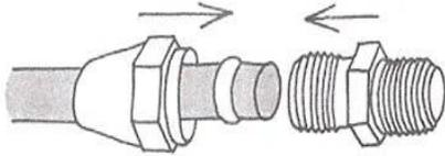
Compression fittings use threaded male and female connections and compression ring, don't require initial flaring.
