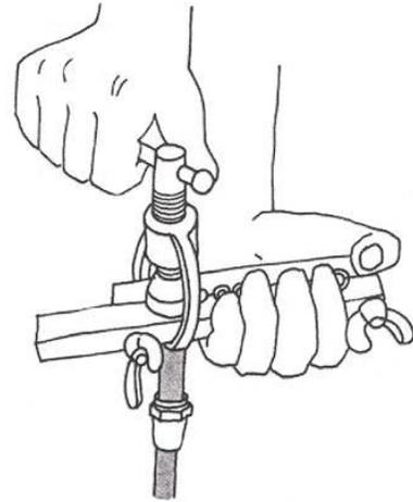
*Special flaring tool does precise job. Clamp it down over pipe end and screw tapered head into pipe, creating flare.*
