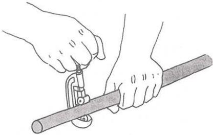
Special pipe cutter for plastic gives good, even cut. Blade on this cutter is narrow to prevent large burrs.
