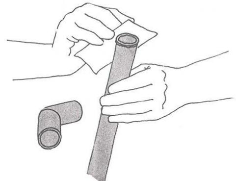
Once you've removed any burrs from inside and outside the pipe end, clean it off very thoroughly with a dry cloth.
