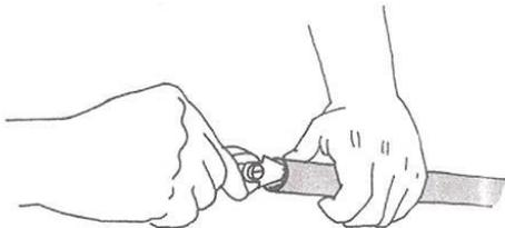
After cutting plastic pipe you'll find burrs, just as on metal. You can remove them with a sharp knife instead of a reamer.
