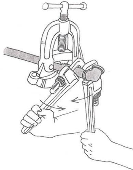
**Step 8.** Use two wrenches to tighten joint—one on pipe, one on fitting. Turn slowly in opposite directions.
