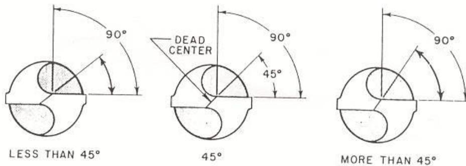
Examples of correct and incorrect angles for sharpening twist drill. (See Figure IX.)
