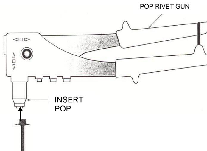
5. Insert the large rivet through both pieces of sheet metal and rivet by closing the handles of the gun together until the stem pops from the rivet.
