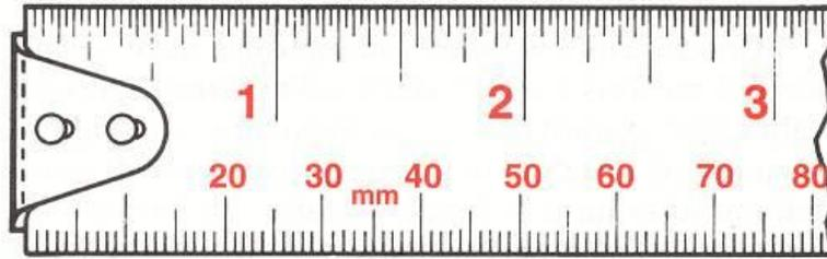
This tape has both U.S. Customary and metric units of measurement. The 1, 2, 3 values refer to inches. The 20, 30, 40 values refer to millimeters.
