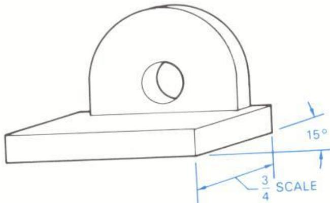
Oblique drawing is a form of pictorial drawing in which the plane of projection is parallel to the front surface of the object. The lines of sight are at an angle to the plane of projection and are parallel to each other. This allows the viewer to see three faces of the object. The front face and any surface parallel to it, is shown in true shape and size, while the other two faces are distorted in relation to the angle and scale used.
