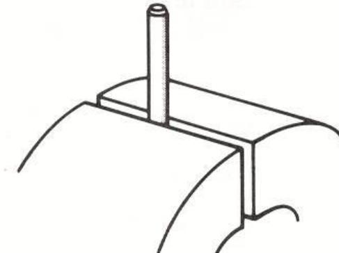
2. Obtain from the instructor a 3/8" - 16NC die and insert it in the die stock so the tapered side of the die will start the threads.
