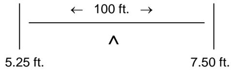
Example:  $7.50 - 5.25$  ft. Difference in elevation = 2.25% slope
