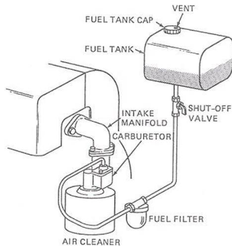
2. Vacu-jet or Suction Feed. This type of carburetor is used when the fuel tank is below the carburetor. It uses the force of atmospheric pressure to move the fuel from the tank to the carburetor. (See Figure X.)
