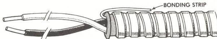
Armored cable consists of two or three wires, protected by a layer of tough paper and flexible aluminum or galvanized steel armor. Note the bonding strip under the armor.
