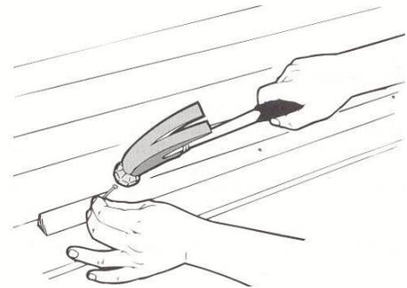
**Proper procedure for grasping hammer:**
