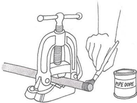
**Step 6.** Threads cut, pipe end cleaned off, apply pipe joint compound to threads to help seal the completed joint.
