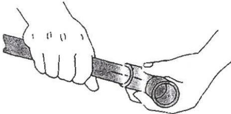
**Place fitting over the end of the pipe (it should fit snugly) and mark both pipe and fitting to show exact placement.**
