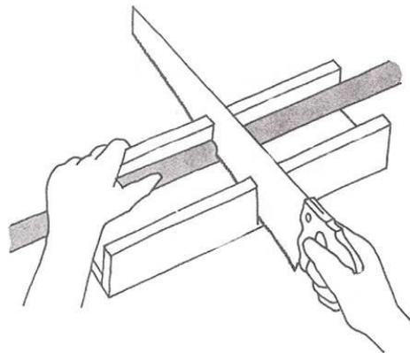
You can also cut plastic pipe with a regular handsaw. To insure a square cut, place it in a miter box, hold securely.
