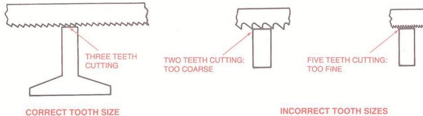
When cutting mild steel or cast iron over 1/8" thick, use a coarse blade (18 teeth per inch). Hard steel, pipe, and heavy sheet metal can be cut with a medium blade (24 teeth per inch). Thin sheet metal tubing should be cut with a fine blade (32 teeth per inch).
