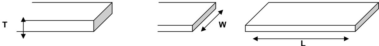
$$\frac{\text{THICKNESS (IN INCHES)} \times \text{WIDTH (IN INCHES)} \times \text{LENGTH (IN FEET)}}{12} = \text{BOARD FEET}$$
