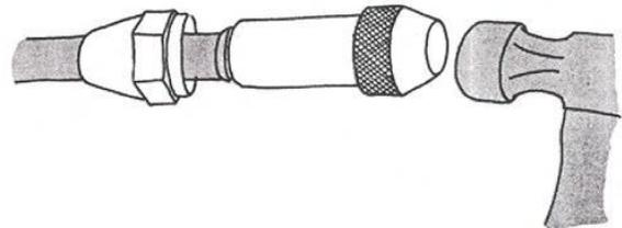
*Tapered end of flaring tool fits into end of pipe, is hammered in to make flare. Use vise for support.*
