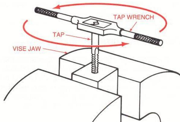
4. Using both hands, grasp the handles and turn slowly using even pressure on the handles to prevent breaking the tap.
